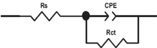
Fig. 6. Equivalent circuits compatible with experimental impedance data.
